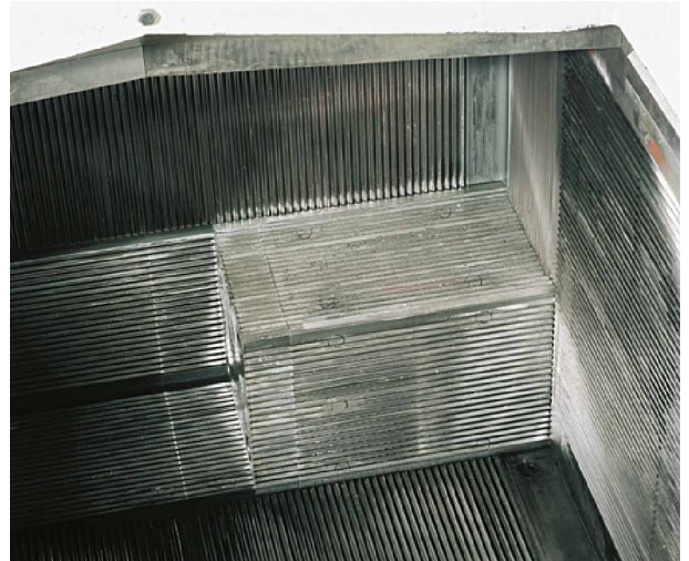
Pic. 2: Wash-board wear plate lining in a scrap baling press type Rapida III
