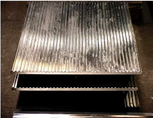
Pic 1: profiled wear plates for scrap baling presses.
