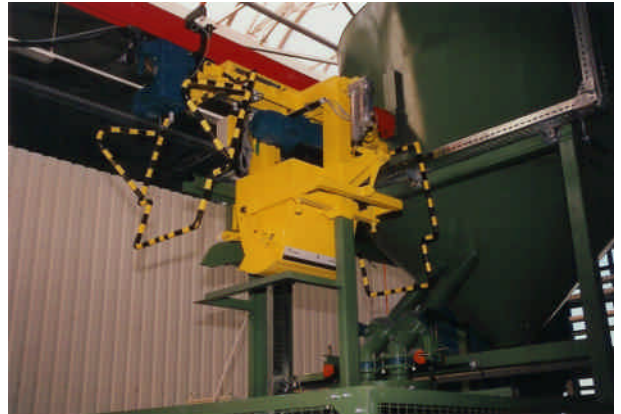
Pic 5: Transfer point from horizontal to vertical bucket transport
