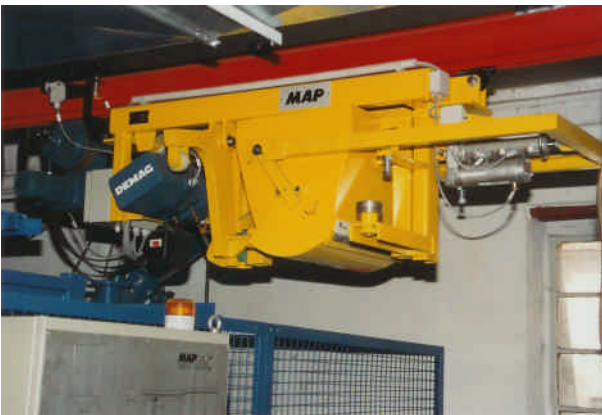
Pic.4: Hoist gear with bucket in flat design
