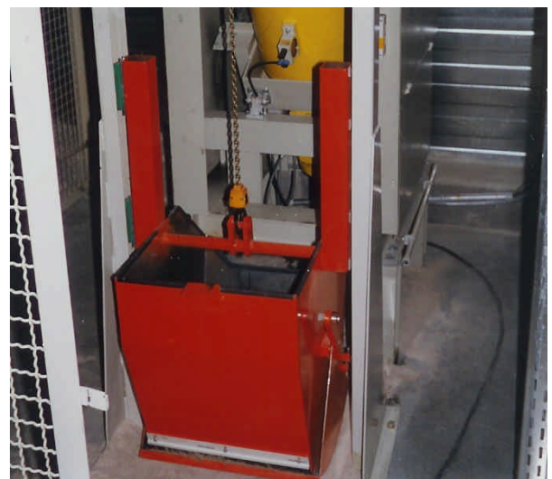
Pic. 2: Bucket with chain hoist in lowered charging position beside the mixer
