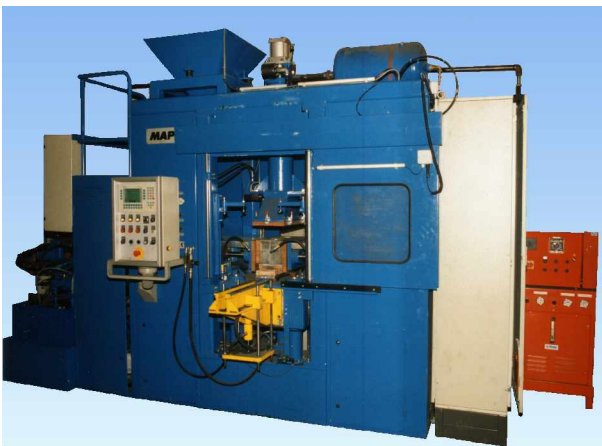
Pic.1: 12 Litre Core Shooter, Type MAP, with gassing unit (red)
