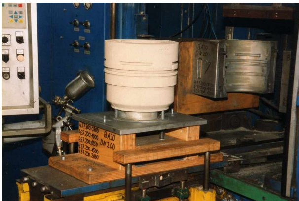
Pic.3: Core shooter with vertical divided core box and pin plate
