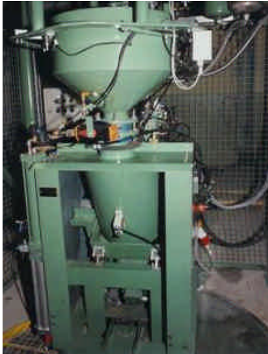
Pic. 3: Mixer with a weighing bin for material dosing
