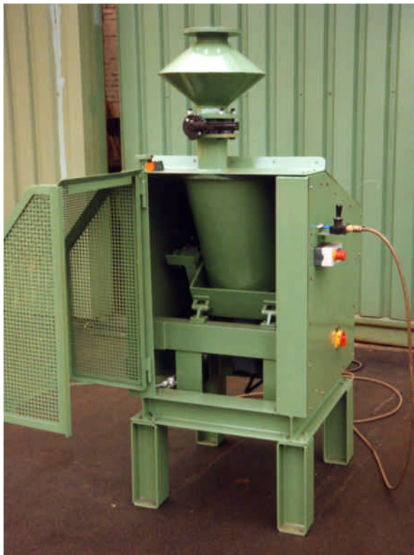
Pic.1: PKM core sand mixer in tilting position, using a volumetric dosing device.
