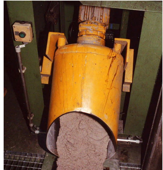
Pic.2: PKM core sand mixer in emptying position on mixer platform
